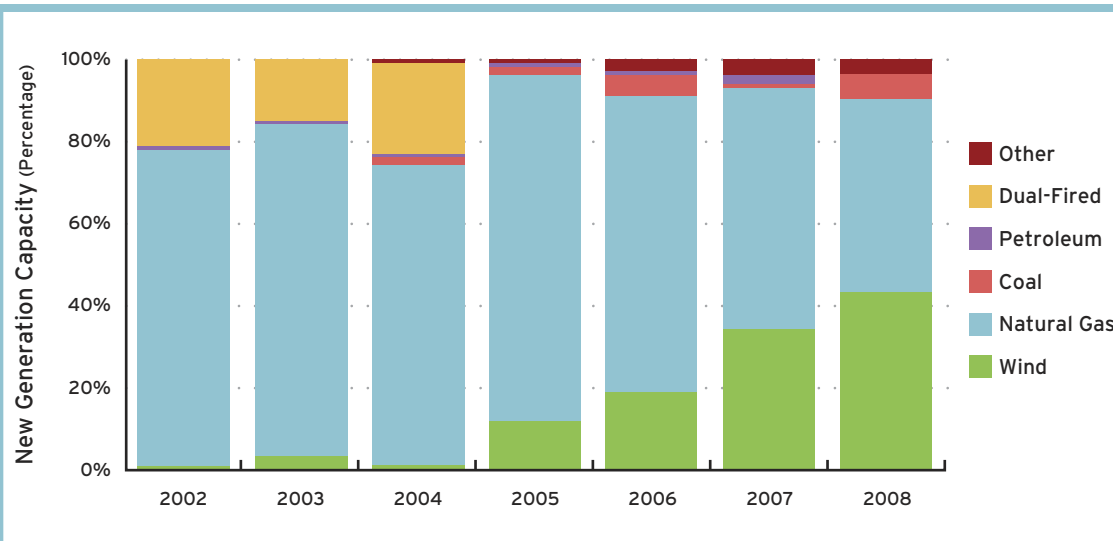
FIGURE 2. New U.S. Generating Capacity by Energy Source Source: Annual Report on U.S. Wind Power Installation, Cost, and Performance Trends: 2007, U.S. Department of Energy 11
